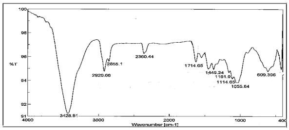
Fig. 26. FT-IR of Bit. /  $AO_1(0.5\%)$  / SBS blend after TFOT .
