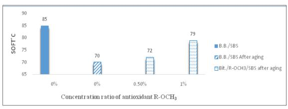
Fig. 13. Softening point of SBSMB at different concentration ratios of  $AO_1$ .
