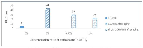
Fig. 15. Ductility of SBSMB at different concentration ratios of AO<sub>1</sub>.
