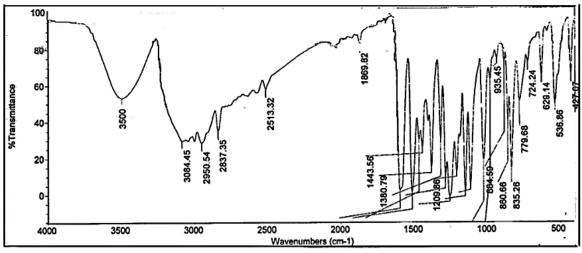
Fig. 2. FTIR of AO<sub>1</sub> antioxidant.
