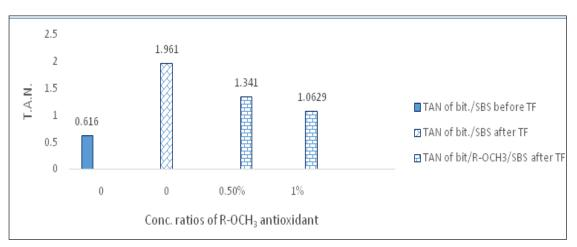
Fig. 30. T.A.N. of Bit. /AO<sub>1</sub>/SBS blends at different concentration ratios of AO<sub>1</sub>.
