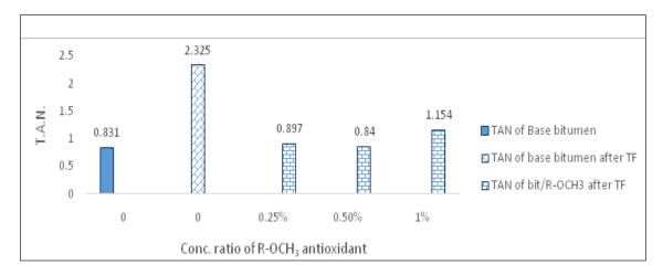
Fig. 28. T.A.N. of Bit. /AO<sub>2</sub> blends at different concentration ratios of AO<sub>2</sub>.
