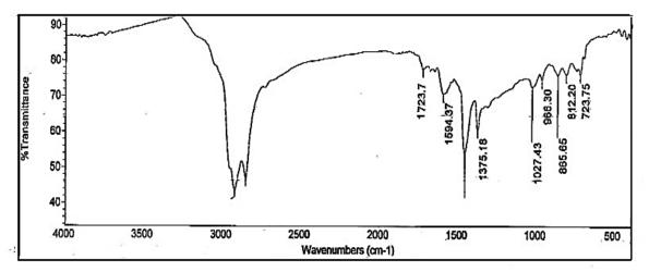
Fig. 24. FT-IR of Bit. /SBS blend before TFOT.
