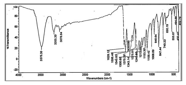
Fig. 3. FTIR of AO<sub>2</sub> antioxidant.
