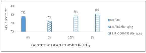
Fig. 12. Viscosity of SBSMB at different concentration ratios of AO1.
