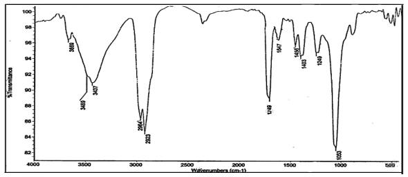
Fig. 17. FT-IR of the base bitumen after TFOT.
