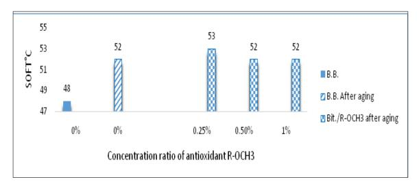
Fig.8. Softening point of bitumen at different concentration ratios of AO<sub>1</sub>.
