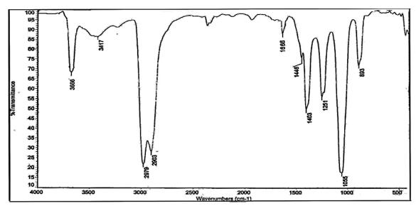
Fig. 16, FTIR of the base bitumen.
