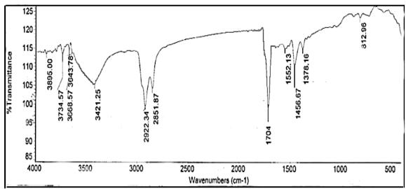
Fig. 23. Effect of (1%) AO<sub>2</sub> on the thermal oxidation of bitumen .
