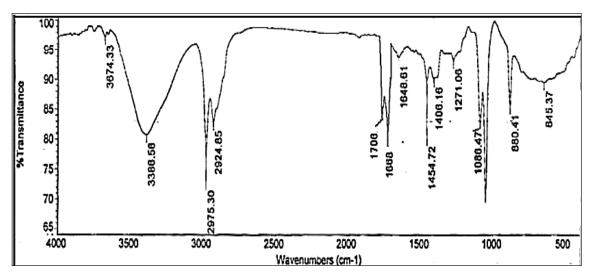
Fig. 22. Effect of (0.5%)  $AO_2$  on the thermal oxidation of bitumen .
