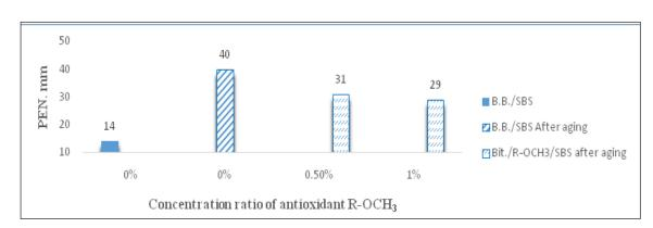
Fig. 14. Penetration of SBSMB at different concentration ratios of AO<sub>1</sub>.
