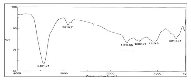
Fig. 27. FT-IR of Bit. /  $AO_{1}(1\%)$  / SBS blend after TFOT .
