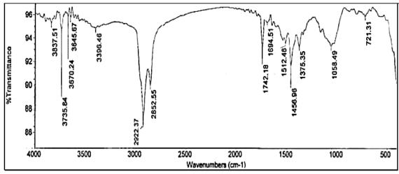
Fig. 25. FT-IR of Bit. /SBS blend after TFOT.
