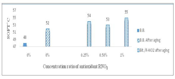
Fig. 9. Softening point of bitumen at different concentration ratios of AO<sub>2</sub>.
