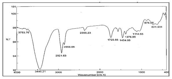
Fig. 20.Effect of (1%)  $AO_1$  on the thermal oxidation of bitumen .
