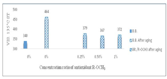
Fig. 6. Viscosity of bitumen at different concentration ratios of AO<sub>1</sub>
