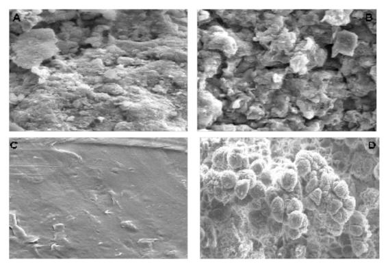
**Fig. 4. SEM of A) Pure MMT, B) Modified MMT, C) Pure PP and D) PP/Modified MMT nanocomposite** *Egypt. J. Chem.* **61**, No.2 (2018)
