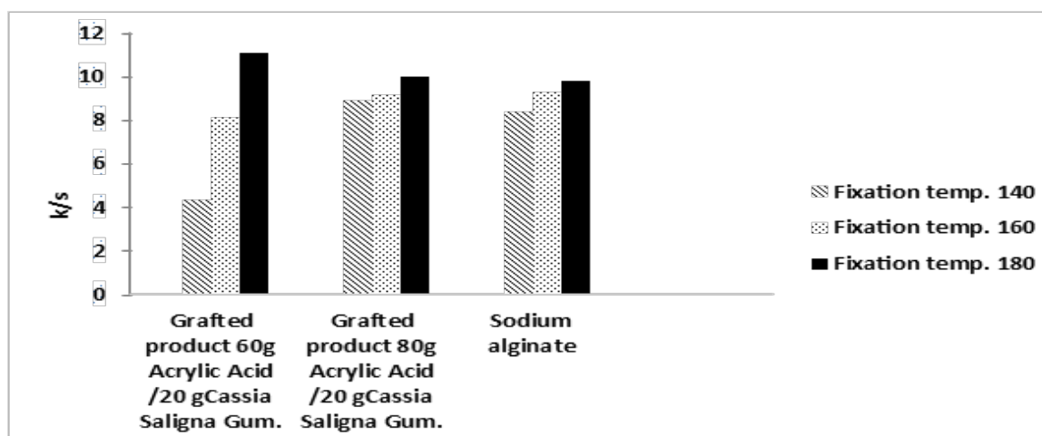
Fig. 2. Color strength of printed cotton fabrics with Tulactive Blue P3R using prepared acrylic acid/cassia saligna gum and commercial sodium alginate as thickeners, and the printing paste stored for 7 days at different fixation temperature.
