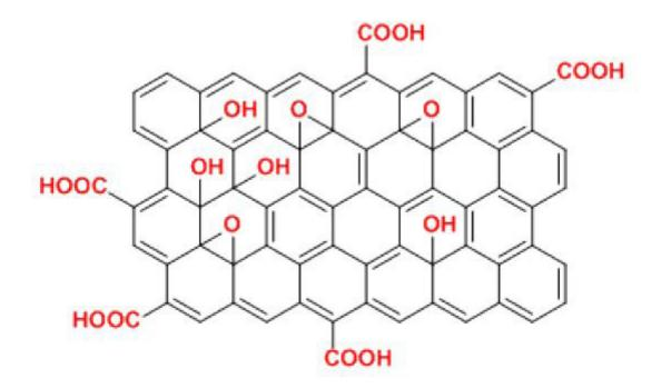
Fig. 4. Schematic structure of graphene oxide (GO) [15].
