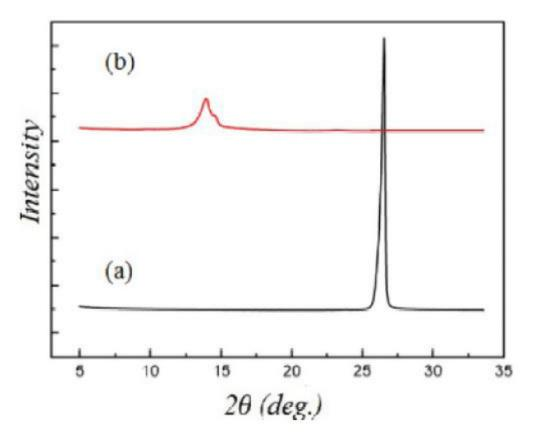
Fig. 7. XRD patterns of graphite (a), graphene oxide (b) [32].
