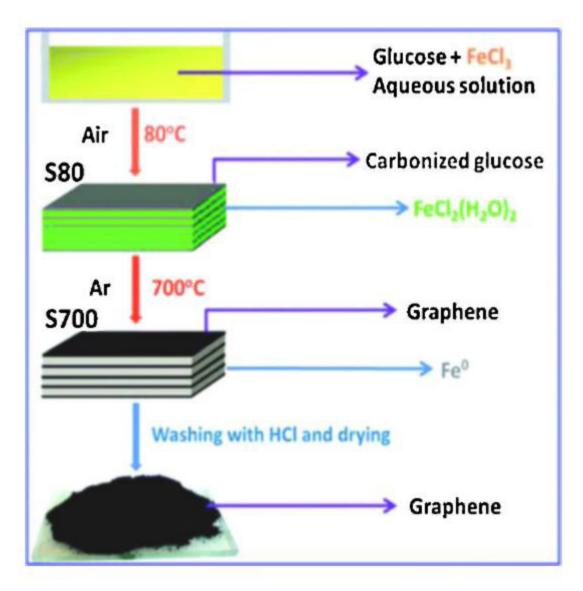
Fig. 6. Schematic representation of graphene preparation with aid of ferric chloride solution [30].
