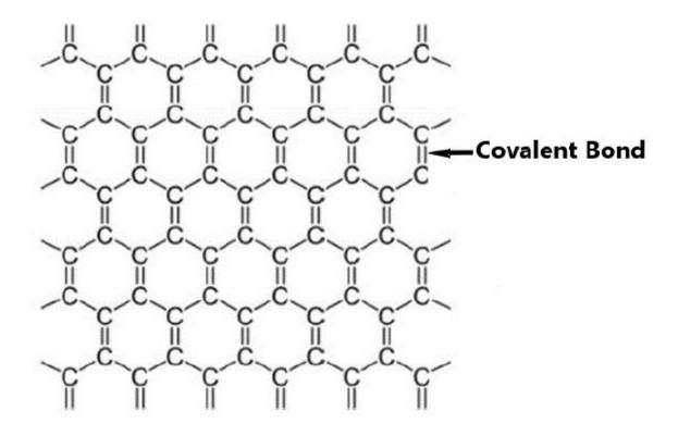
Fig. 3. Graphene structure.
