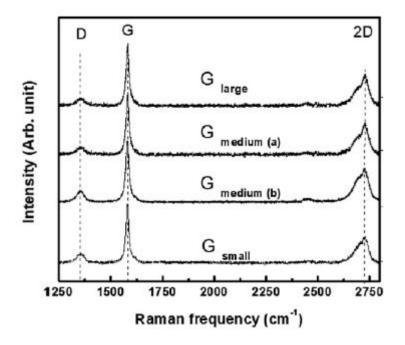
Fig. 9. Raman spectroscopy of graphene oxide [38].
