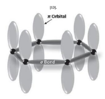
Fig. 2. The sp<sup>2</sup> hybridization between carbon atoms and formation of  $\pi$  bonds from the unoccupied p-orbital
