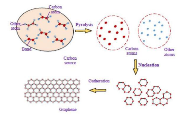
Fig. 5. Mechanism of thermal method for growing of graphene [21].
