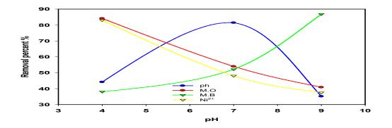
Fig. 3. Effect of medium pH on removal percent of pollutants at initial concentration; 100 ppm, dose; 1g, Temperature; 80°C, and contact time; 150 min.
