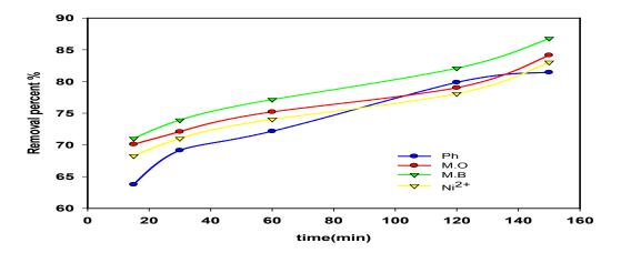
Fig. 4. Effect of time on removal percent of pollutants at initial concentration; 100 ppm, medium pH;4 for (Ni2+,MO), 9 for (MB), 7 for (Ph) Temperature; 80°C and dose;1g
