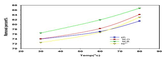
Fig. 9. Effect of temperature on the removal percent of pollutants at initial concentration;100ppm, at contact time; 150min., medium pH; 4 for (Ni<sup>2+</sup>, MO), 9 for (MB),7 for (Ph) and adsorbent dose; 1g.
