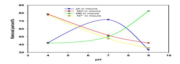
Fig. 11. Effect of medium pH on removal percent of pollutants in mixture at initial concentration; 100 ppm, dose; 1g, Temperature; 80 °C, and contact time;150 min.
