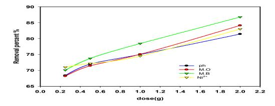
Fig. 6. Effect of adsorbent dose on removal percent of pollutants at initial concentration; 100ppm, medium pH; 4 for (Ni<sup>2+</sup>,MO), 9 for (MB), 7 for (Ph) Temperature; 80°C, and contact time; 150min.
