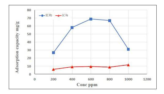
Fig. 5. Effect of concentration of Pb (II) and Fe (II) on the adsorption capacity
