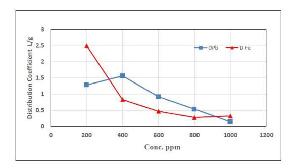
Fig. 6. Effect of concentration of Pb (II) and Fe (II) on the distribution coefficient
