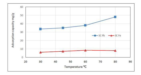
Fig. 8. Effect of temperature on the adsorption capacity of Pb (II) and Fe (II)
