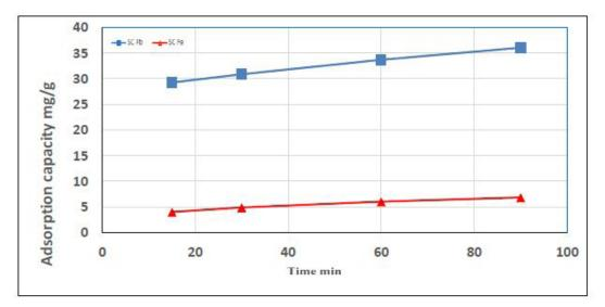
Fig. 11. Effect of contact time on the adsorption capacity of Pb (II) and Fe (II)
