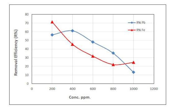
Fig. 4. Effect of concentration of Pb(II) and Fe(II) on the removal efficiency
