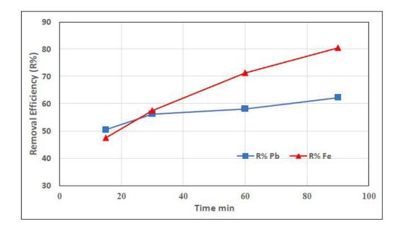
Fig. 10. Effect of contact time on the removal efficiency of Pb (II) and Fe (II)
