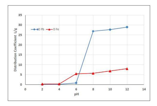
Fig. 3. Effect of pH on the distribution coefficient of Pb (II) and Fe (II)
