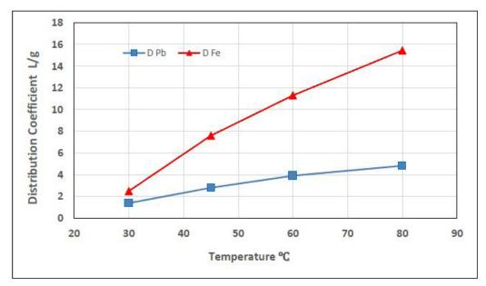
Fig. 9. Effect of temperature on the distribution coefficient of Pb (II) and Fe (II)
