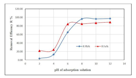
Fig. 1. Effect of pH of adsorption solution on the removal efficiency of Pb (II) and Fe (II)
