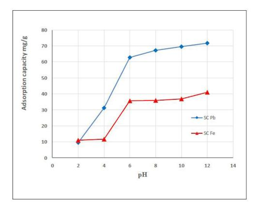
Fig. 2. Effect of pH on the adsorption capacity of Pb (II) and Fe (II)
