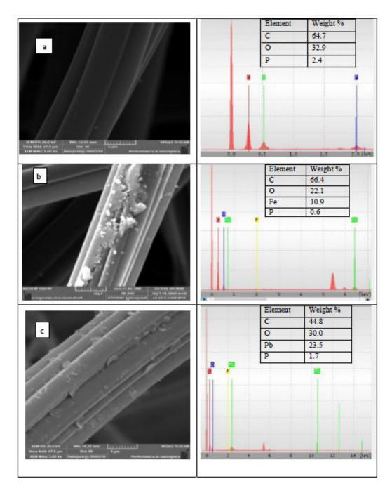
Fig. 13. SEM Micrographs and EDX of ACF. (a) Blank sample of ACF, (b) ACF after Fe(II) adsorption, and (c) ACF after Pb(II) adsorption.
