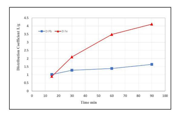
Fig. 12. Effect of time on distribution coefficient of Pb (II) and Fe (II)
