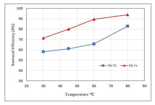
Fig. 7. Effect of temperature on the removal efficiency of Pb (II) and Fe (II)
