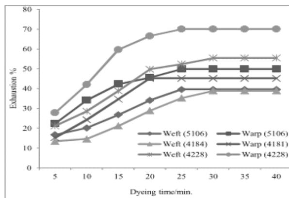
Fig.2. Sorption rate of Suncron Orange 3 for the different polyester fabric at 80°C.
