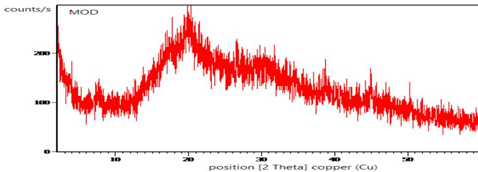
**Fig. 1. X-ray diffraction of modified chitosan.**
