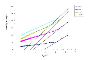
Fig. 3. Energies gaps for allowed indirect transition of PVA/SiO<sub>2</sub> nanocompsites.
