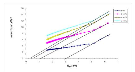
Fig. 4. Energies gaps for forbidden indirect transition of PVA/SiO, nanocompsites.
