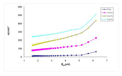
Fig. 2. Effect of silicon dioxide nanoparticles concentrations on the absorption coefficient of PVA .
