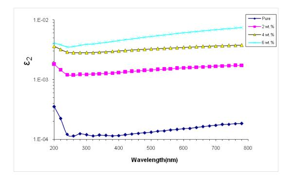
Fig. 8. Variation of imaginary part of dielectric constant for PVA/SiO2 nanocomposites with photon wavelength.
