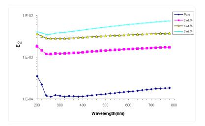
Fig. 7. variation of real part of dielectric constant for PVA/SiO, nanocomposites with photon wavelength.
