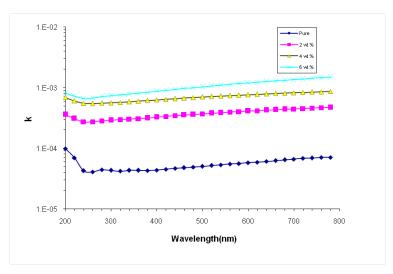
Fig. 5. Variation of the extinction coefficient with the incident photon wavelength of (PVA-SiO<sub>2</sub>) nanocomposites.
