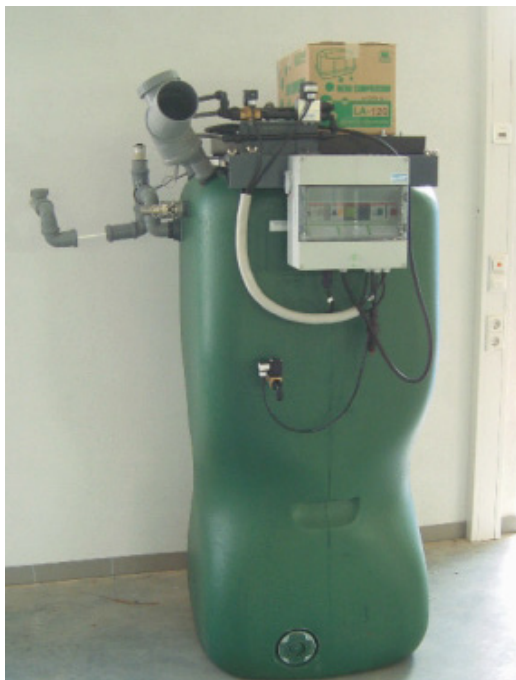
Fig. 14. The MBR pilot unit for the treatment of blackwater in Egypt [4].
