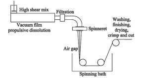
Scheme (4): Dry jet wet spinning in lyocell process.
