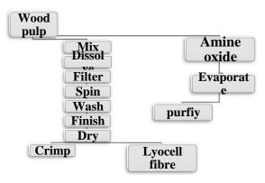
Scheme (5): Manufacture process for the lyocell fibers
