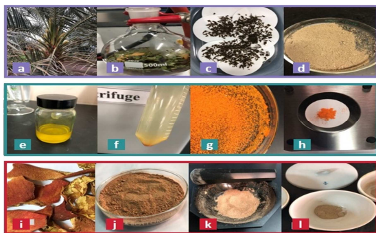
Figure 1: Isolation of cellulose acetate from Palm Branch (a-c), cellulose Acetate (d), Synthesis of nano CUR (e-h), Synthesis of Ag NPs (i-l)
