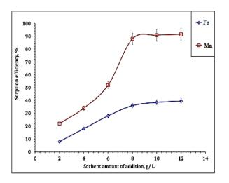
Fig. 6. Effect of adsorbent amount upon Fe (III), Mn(II) adsorption efficiency onto B- 8 (PH 3, 12 h, and room temperature)
