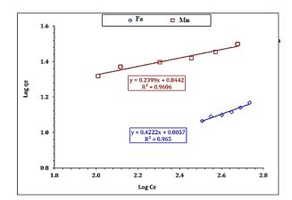
Fig. 4. Freundlich line plans for sorption of Fe (III), Mn(II) onto B-8.
