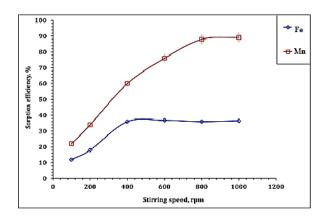
Fig. 7. Influence of agitation moving rpm on Fe (III), Mn(II) sorption effectiveness % (10 h, 0.12 / 15 g/ mL, ( $\approx 25$  °C).
