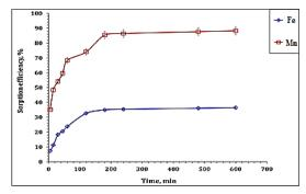
Fig. 1. Influence of the contact time on Fe (III), Mn(II) adsorption efficiency by (B- 8) (0.12 g/15 ml,100 mg/L at  $\approx$  25 °C and pH 2.9
