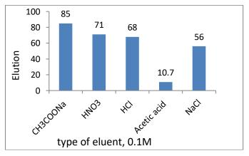
Fig.8: Elution yields using different eluent reagents
