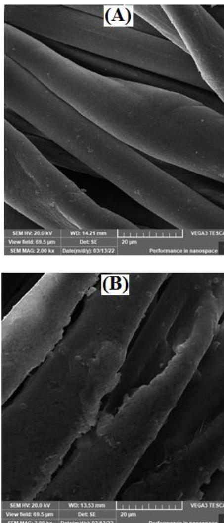
**Fig. 6.** SEM images of untreated fabric (A) and PDMS emulsion (40 g/L) treated fabric (B).
