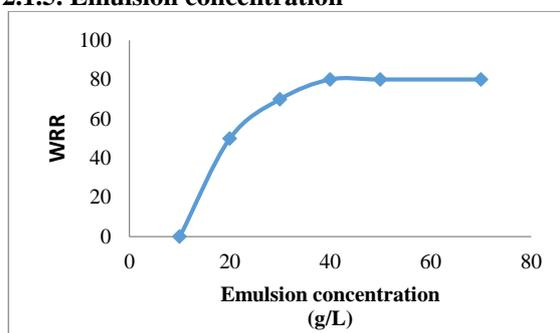
**Fig. 3.** Effect of emulsion concentration on WRR of treated fabric. The PDMS emulsion ingredients: PDMS (5%); TEA (2.4%); SA (4.5%); and AlCl<sub>3</sub>/SA molar ratio 1. The fabric is treated with different emulsion concentrations and then dried at 100 °C/5min.
