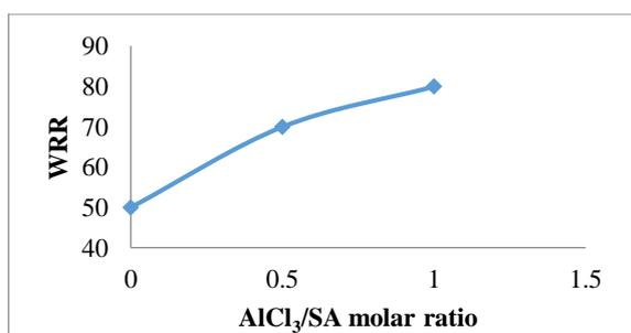
**Fig. 2.** Effect of AlCl<sub>3</sub>/SA molar ratio on WRR of treated fabric. The PDMS emulsion ingredients: PDMS (5%); SA (4.5%) and TEA (2.4%). The fabric is treated with 50 g/L of mother emulsion and then dried at 100 °C/5min.
