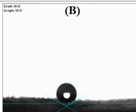
**Fig. 8.** Images of water droplets on surface of the water repellent fabric samples treated with the PDMS emulsion (40 g/L) and then dried at 100 °C (A) or 160 °C (B).
