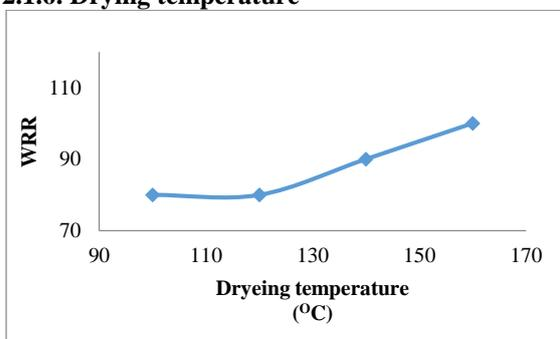
**Fig. 4.** Effect of drying temperature on WRR of treated fabric. The PDMS emulsion ingredients: PDMS (5%); SA (4.5%); TEA (2.4%) and AlCl<sub>3</sub>/SA molar ratio (1/1). The
