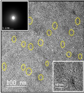
Fig. 6.TEM image of red-emissive CDs; upper inset: electron diffraction pattern, lower inset: high magnification).
