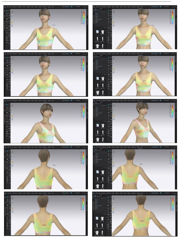
Figure 4: *CLO3D* Simulation System for evaluation of fitting and stretch-ability of sample number 7 (light weight 92/8 knitted PET/L blended fabric)
