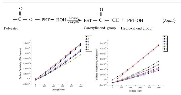
**Fig. 2:** Surface resistivity of untreated (left) and bio-treated (right) knitted PET/L blended fabrics with different blending ratios
