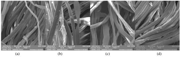
Figure 3: Scanning electron micrographs of untreated and bio-treated PET/L knitted fabric. (a) untreated sample number 7, (c) untreated sample number 8, (b) bio-treated sample number 7, and (d) bio-treated sample number 8
