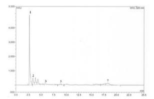
Fig. (7): HPLC chromatogram of alcoholic extract of *T*. myriocarpa
