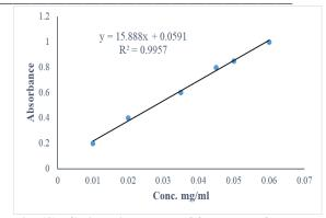
Fig. (2): Calibration curve of ferrous sulfate standard
