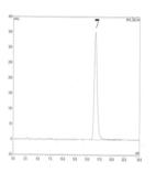
Fig. (16): HPLC chromatogram of ferulic acid standard
