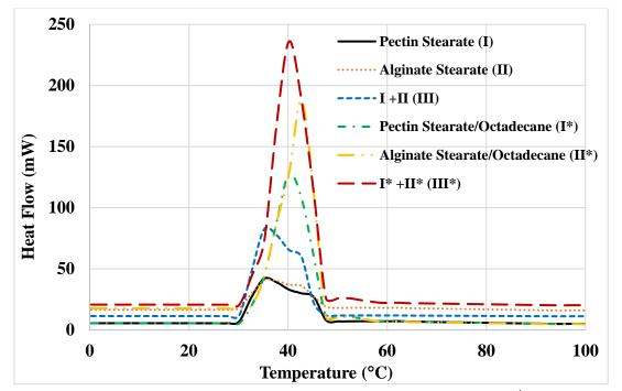
Figure 2: DSC curves for hosting materials with/without Octadecane from 2<sup>nd</sup> heating
