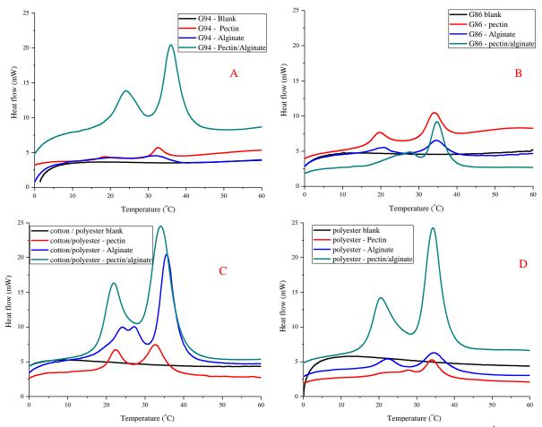
Figure 3: DSC curves for covered yarns with pectin or alginate/stearic acid and Octadecane at 2<sup>nd</sup> heating a) Cotton G94, b) Cotton G86, c) Cotton G86/polyester, and d) Polyester
