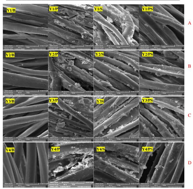
Figure 4: SEM of different yarn materials after applying PCMs treatments (A) Cotton G 94, (B) Cotton G 86, (C) Cotton G86 /Polyester and (D) Polyester
