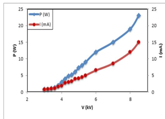
Fig. 4. The relation between the discharge power (P) and the current (I) as a function of the discharge voltage (V) at fixed oxygen rate.
