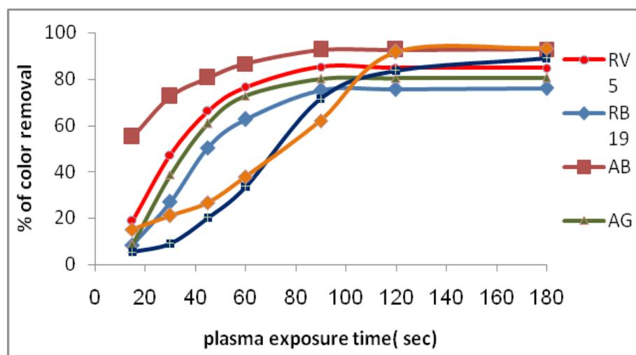
Fig. 8. The effect of plasma exposure time on the percent of color removal for the six dyes.
