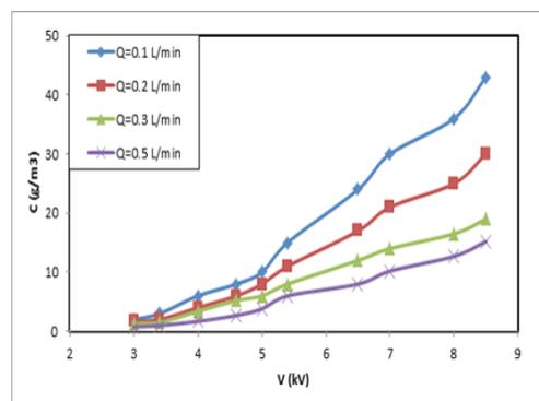
Fig. 5. The ozone concentration as a function of the discharge voltage at different oxygen flow rates.
