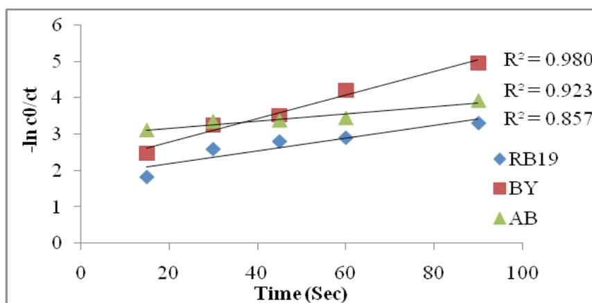
Fig. 12. Decolorization kinetics of RB19, BY&AB dyes solution at different plasma exposure time (sec).
