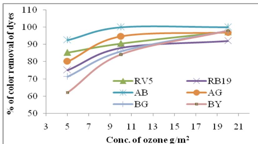
Fig. 9. The effect of ozone concentration on the % of color removal for the six dyes.
