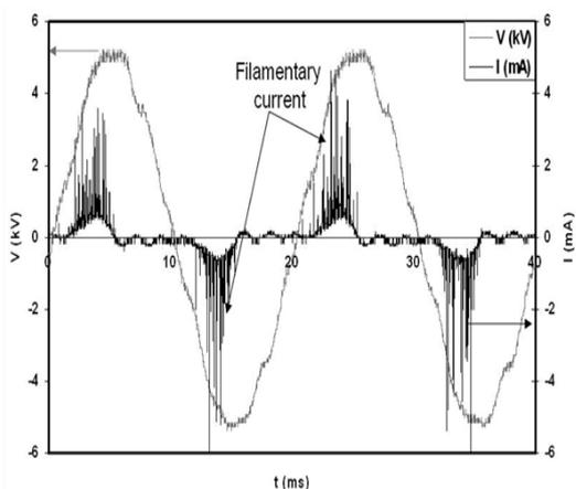
Fig. 3. Voltage and current wave resulting from DBD.
