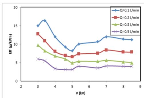
Fig. 6. The ozone efficiency as a function of the discharge power at different oxygen flow rates.
