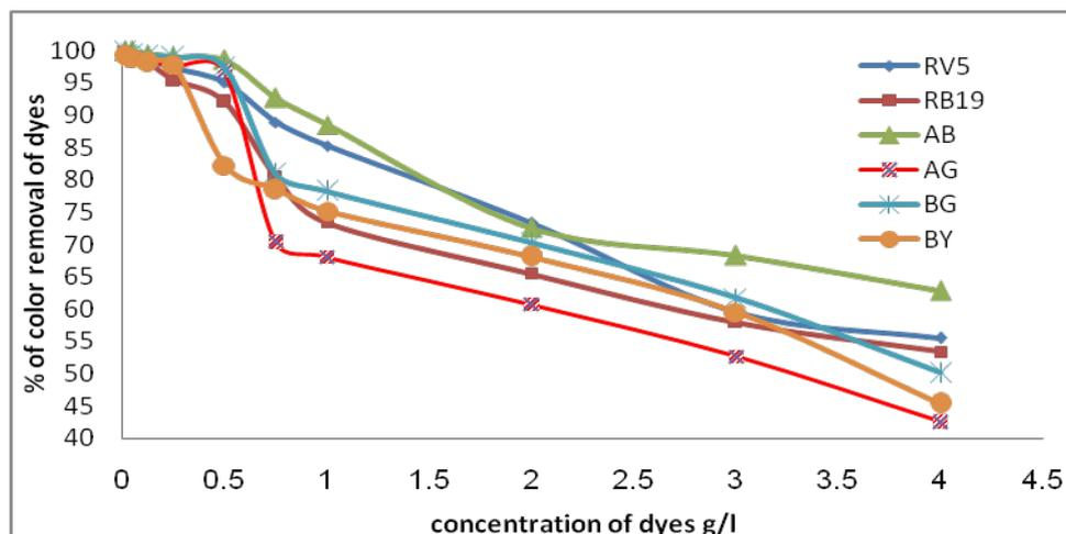
Fig. 10. The effect of dye concentration on the % of color removal for the six dyes.
