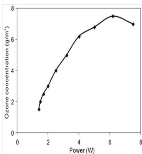
Fig. 7. Ozone concentration in the exhaust gas of the DBD cell as a function of the discharge power.
