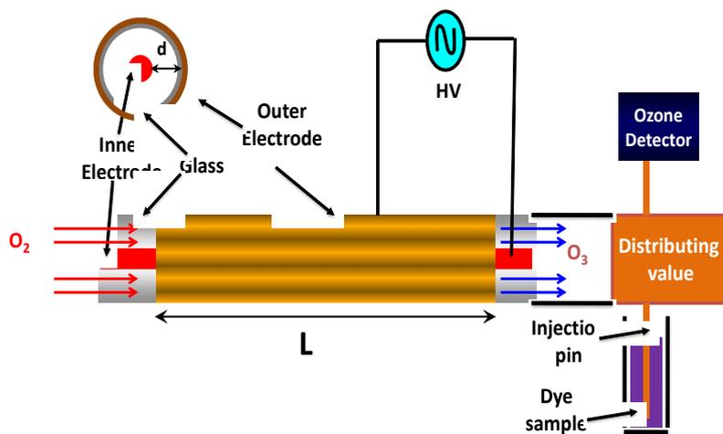
Fig. 1. DBD- plasma ozone- generator scheme.
