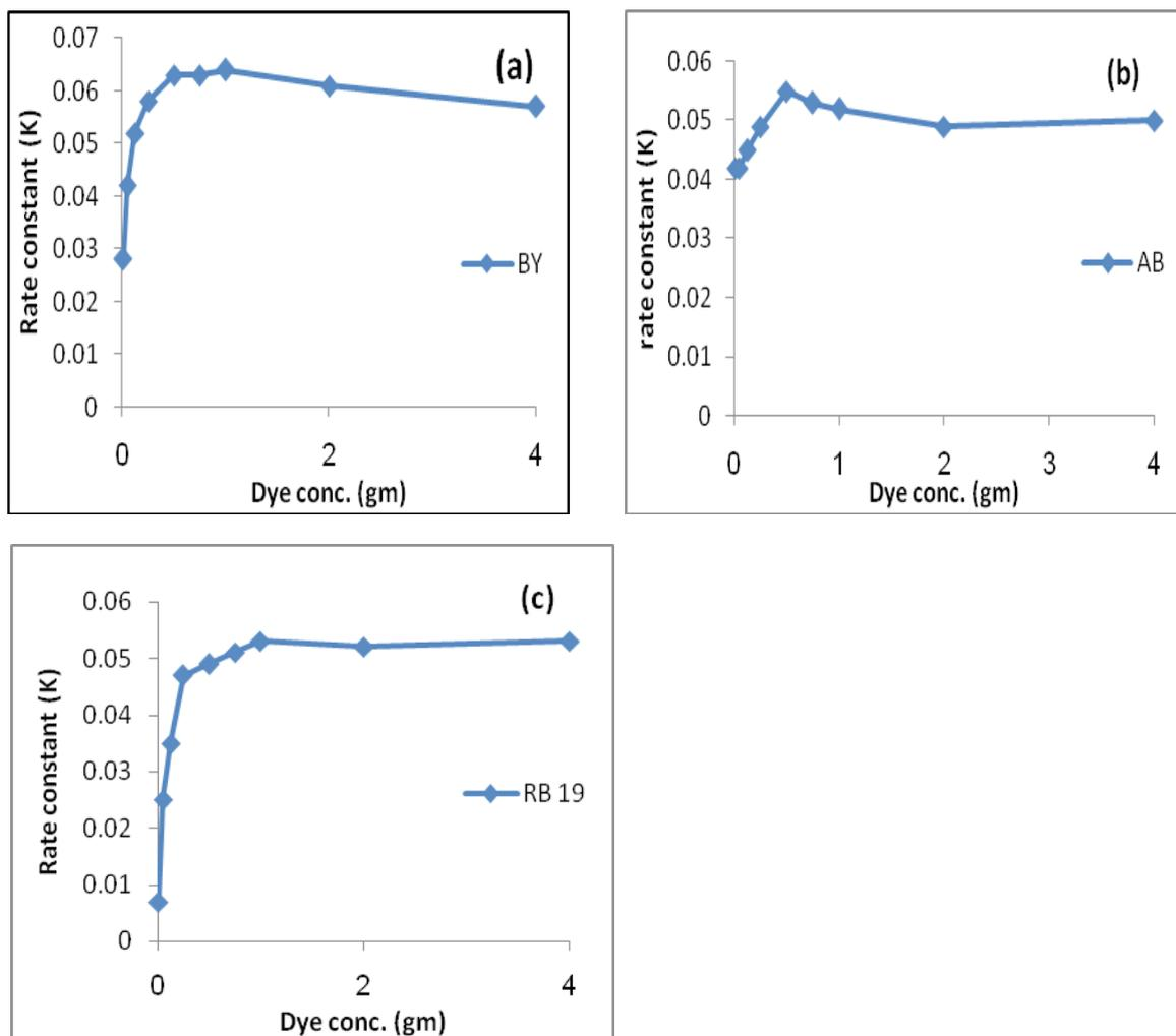
Fig. 11. Effect of concentration of dyes on rate constant  $k$ .
