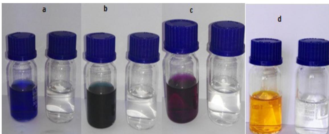
Fig. 2. Colors of the dye solutions (dye concentration 4 g/l) before and after ozone treatment
