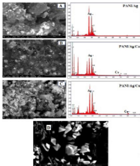
Fig. 3. EDS and SEM micrograph of (A) PANI/Ag, (b) PANI/Ag/Co, (C) PANI/Ag/Cu and (d) PANI.
