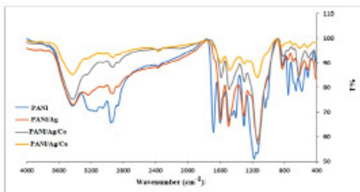
Fig. 2. FT-IR of the prepared pure PANI and PANI nanocomposites.
