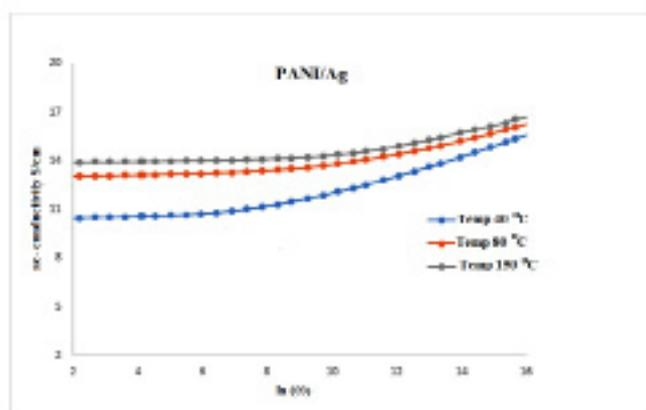
Fig. 4. The variation of ac conductivity with angular frequency at high temperatures.
