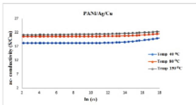
Fig. 6. The variation of ac conductivity with angular frequency at high temperatures.
