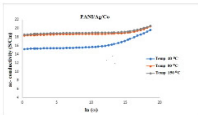
Fig. 5. The variation of ac conductivity with angular frequency at high temperatures.
