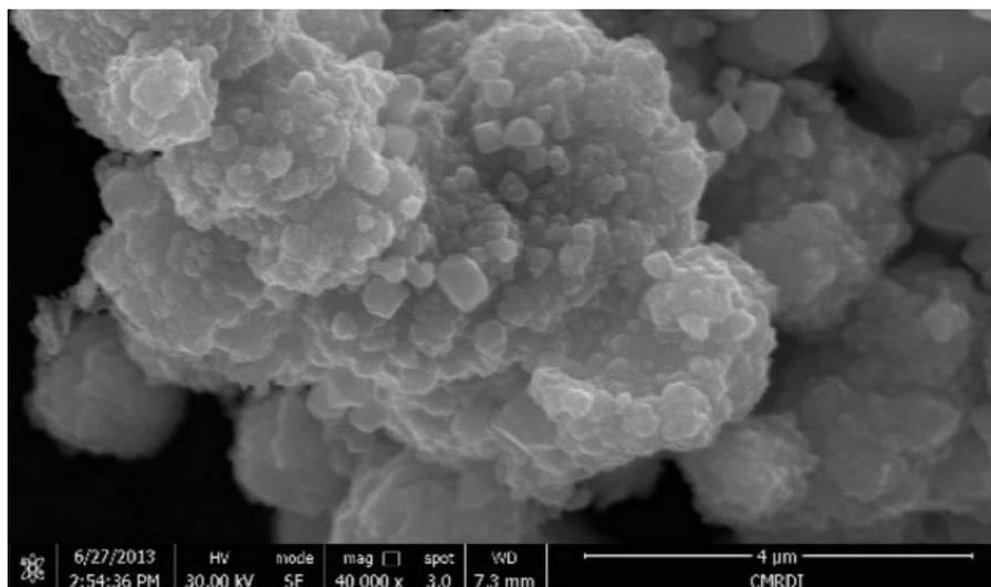
Fig. 1. Scanning electron image of the copper powder prepared by electroless deposition.
