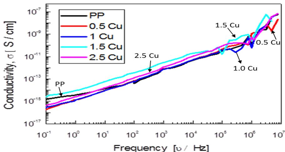
Fig. 6. The electrical conductivity ( $\sigma$ ) of PP/nano-copper composite materials
