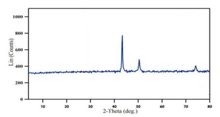
Fig. 2. X-ray diffraction pattern of copper powder.
