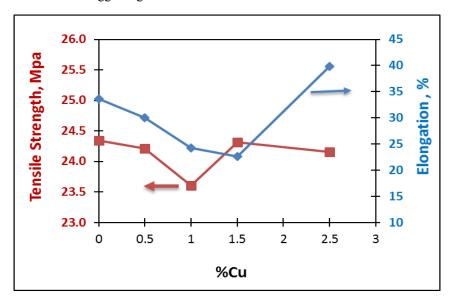
Fig. 8. The tensile strength and elongation variation for PP/nano-copper composite materials.
