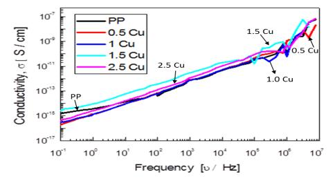
Fig. 6. The electrical conductivity ( $\sigma$ ) of PP/nano-copper composite materials
