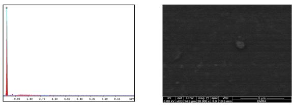
Fig. 3. the SEM and EDAX of pure PP.
