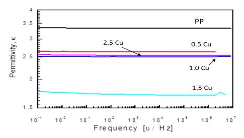
Fig. 5. The dielectric permittivity of PP and PP/nano-copper composite materials.
