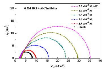
Fig. 4. EIS Nyquist for Zinc in 0.5 M HCl in the absence and presence of different concentrations of AIC, at 298 K.
