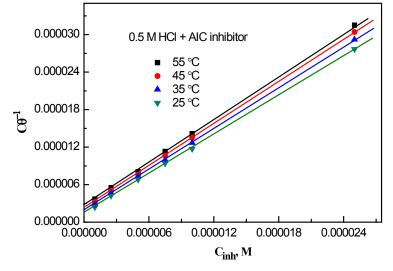
Fig. 8. Langmuir adsorption of AIC inhibitor on Zn in 0.5 M HCl, at different temperatures.
