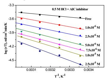
Fig. 7. Transition state plots, variation of log rcorr/T against T-1, for Zn in 0.5 M HCl devoid of and containing different concentrations of AIC.
