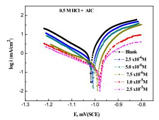
Fig. 3. E-log i curves of zinc in 0.5 M HCl solution in the absence and presence of different concentrations of AIC, at 298 K.
