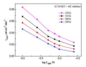
Fig. 2. Variation in the rate of  $H_2$  gas production,  $r_{corr}$ , with the logarithm of AIC concentration, at different temperatures.
