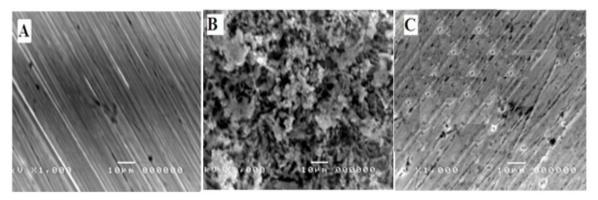
Fig. 10. SEM micrographs of Zn surface (A) polished and after inundation in (B) 0.5M HCl and (C) in 0.5M HCl + 1x10<sup>-5</sup> M AIC inhibitor, for a period of 1 hr, at 25 °C.
