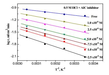
Fig. 6. Arrhenius plots variation of log  $r_{corr}$  against T<sup>-1</sup>, for Zn in 0.5 M HCl devoid of and containing different concentrations of AIC.
