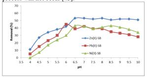
**Figure 3**:Effect of pH on Zn(II), Pb(II) and Ni(II) removal on SB (initial conc. 15 ppm, time 60 min for Zn(II) and Ni(II) and 100 min for Pb(II), dose 0.3 g for Zn(II), 0.1g for Pb(II) and 0.2 g for Ni(II))
