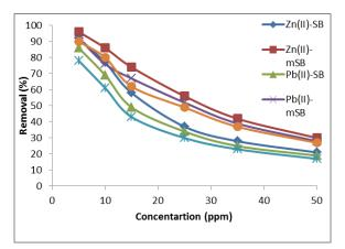
**Figure 6:** Effect of concentration on Zn(II), Pb(II) and Ni(II) removal on SB and mSB (time 60 min for Zn(II) and Ni(II) and 100 min for Pb(II), pH 6.5 for Zn(II) and Ni(II) and 6 for Pb(II), dose 0.3 g for Zn(II), 0.1g for Pb(II) and 0.2 g for Ni(II)).
