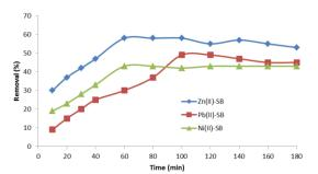
**Figure4:** Effect of contact time on Zn(II), Pb(II) and Ni(II) removal on SB (initial conc. 15 ppm, pH 6.5 for Zn(II) and Ni(II) and 6 for Pb(II), dose 0.3 g for Zn(II), 0.1g for Pb(II) and 0.2 g for Ni(II))
