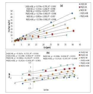
**Figure 7:** Langmuir (a) and Freundlich (b) models of Zn(II), Pb(II) and Ni(II) adsorption on SB and mSB.
