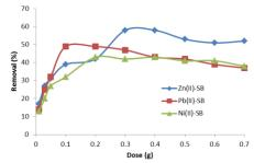
**Figure 5**: Effect of dose on Zn(II), Pb(II) and Ni(II) removal on SB (initial conc. 15 ppm, time 60 min for Zn(II) and Ni(II) and 100 min for Pb(II), pH 6.5 for Zn(II) and Ni(II) and 6 for Pb(II)).
