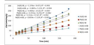
**Figure 8:** Pseudo-second-order kinetic model of Zn(II), Pb(II) and Ni(II) adsorption onSB and mSB.
