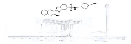
Figure (5): <sup>1</sup>H-NMR of Synthesized 5a Dye.
