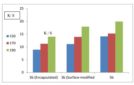
**Figure (16):** Effect of Inkjet Printing Temperature on The Color Strength of Inkjet Printed Polyamide Fabric Using dyes 3b and 5<sub>b</sub>, Fixation Time 2 min.
