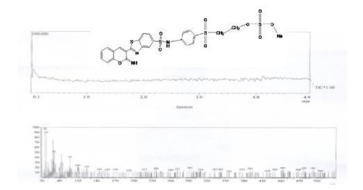
Figure (9): Mass Spectra of Synthesized 5b Dye.
