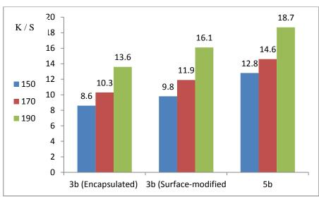
Figure (15): Effect of Inkjet Printing Temperature on The Color Strength of Inkjet Printed Polyester Fabric Using dyes 3b and  $5_b$ , Fixation Time 2 min.
