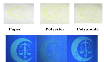
Figure (12): Luminescence Logo of the Printed dye 3b (Micro- encapsulation) without and under UV illumination (365 nm).
