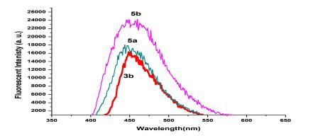
Figure (10): Fluorescence Spectra of 3<sub>b</sub> and 5<sub>a and b</sub> Dye.
