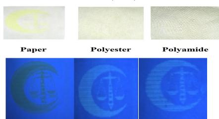
Figure (13): Luminescence Logo of the Printed dye 3b (Surface modified) without UV illumination and under UV illumination (365 nm).
