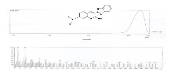
Figure (7): Mass Spectra of Synthesized 3b Dye.
