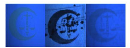
Figure (14): Luminescence Logo of the Printed dye 5<sub>b</sub> (Surface modified) without UV illumination and under UV illumination (365 nm).
