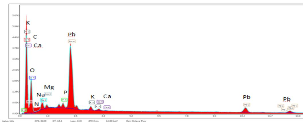
**Fig. 2. Chemical composition of CRBR after adsorption by using EDXA analysis**
