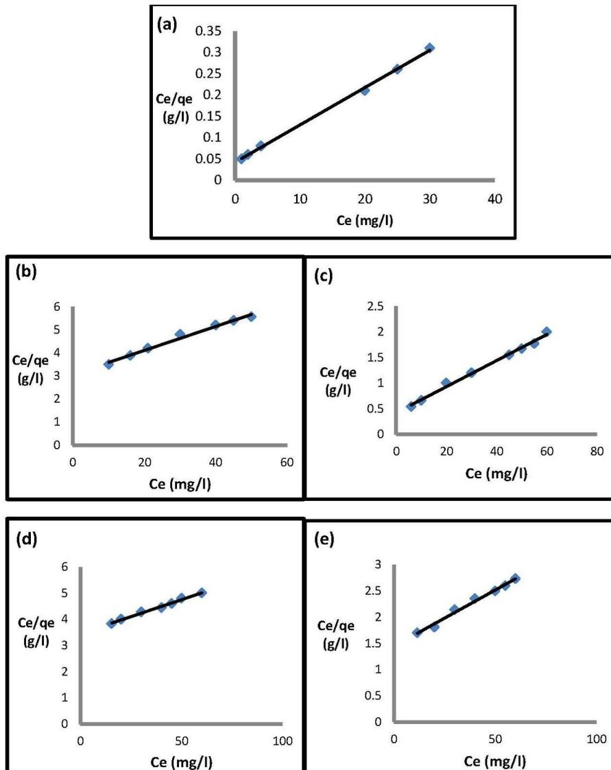
**Fig. 8.** Langmuir plots of MB adsorption onto : a) MWCNTs, b) o-Toluidine, c) MWCNTs/nanocomposite (o-Toluidine), d) m-Toluidine, e) MWCNTs/nanocomposite (m-Toluidine).
