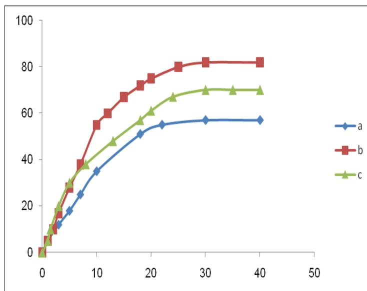
**Fig. 7.** Adsorption isotherm for Pb<sup>2+</sup> onto (a) MWCNTs (b) MWCNTs/nanocomposite (o-Toluidine) and (c) MWCNTs/nanocomposite (m-Toluidine).
