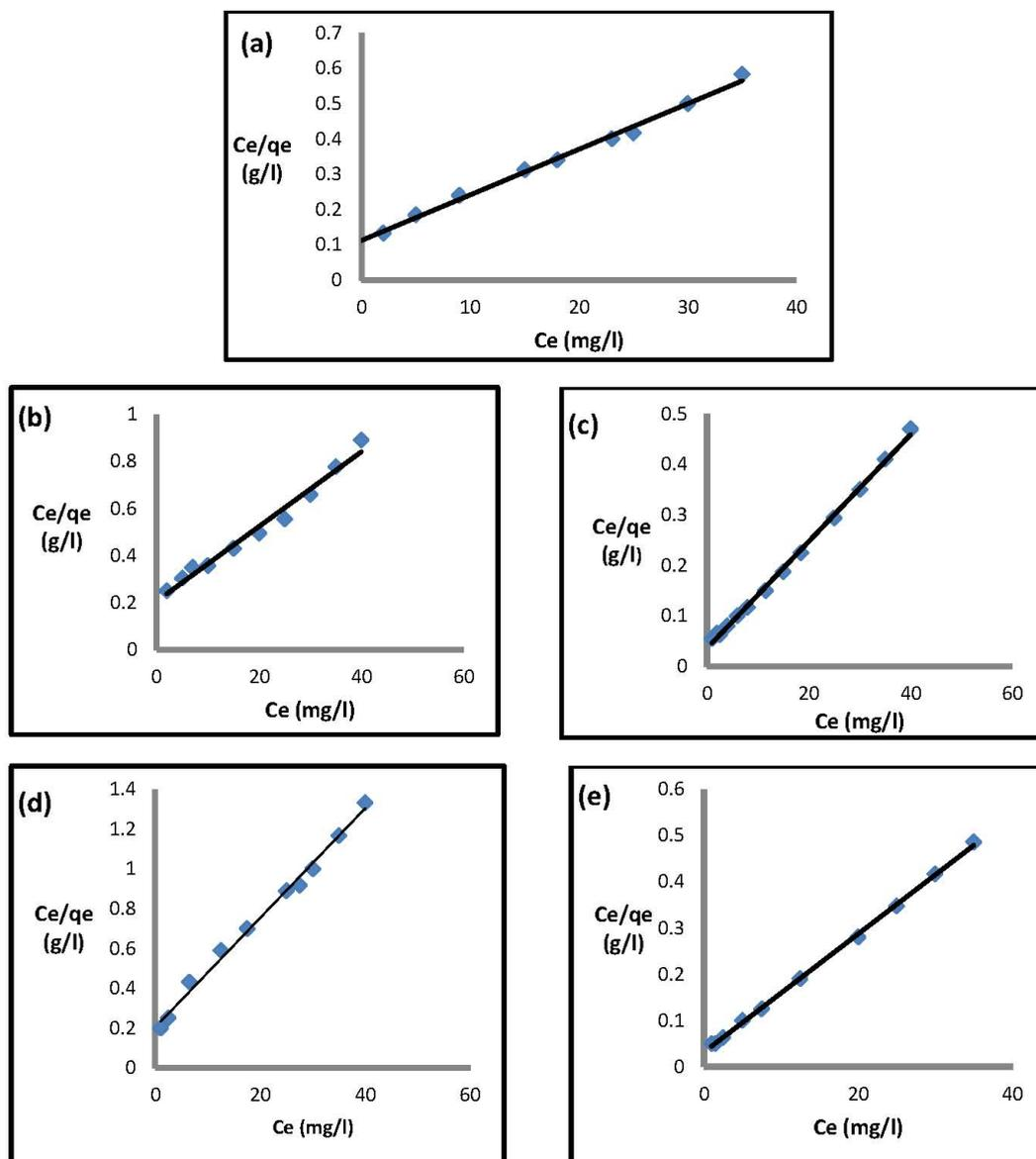
Fig. 9. Langmuir plots of  $Pb^{2+}$  adsorption onto: a) MWCNTs, b) o-Toluidine, c) MWCNTs/nanocomposite (o-Toluidine), d) m-Toluidine, e) MWCNTs/nanocomposite (m-Toluidine).
