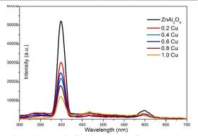
Fig. 11.PL of  $Cu_{(x)}Zn_{(1-x)}$  Al<sub>2</sub>O<sub>4</sub>, nano-powders (where x = 0.0, 0.2, 0.4, 0.6, 0.8, 1.0) using coprecipitation method loaded with carbon spheres
