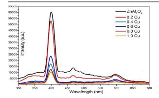
Fig. 10 PL of  $Cu_{(x)}Zn_{(1-x)}$  Al<sub>2</sub>O<sub>4</sub>, nano-powders (where x = 0.0, 0.2, 0.4, 0.6, 0.8, 1.0) by using co-precipitation method non-loaded with CSs
