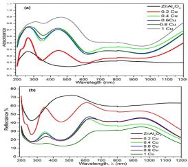
Fig.6: (a) Absorbance (b) Reflectance of Cu<sub>(x)</sub>Zn<sub>(1-</sub> x) Al<sub>2</sub>O<sub>4</sub>, nano-powders (where x = 0.0, 0.2, 0.4, 0.6, 0.6, 0.6, 0.6)
