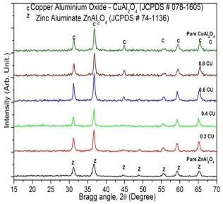
**Fig.2** XRD patterns of  $Cu_{(x)}Zn_{(1-x)}$  Al<sub>2</sub>O<sub>4</sub> (*x* from 0.0 to 1.0 molar ratios) using co-precipitation and loaded with carbon spheres
