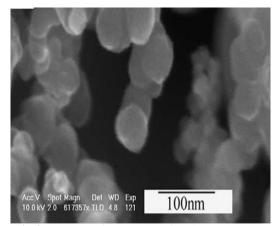
Fig.3 FESEM micrographs of carbon sphere
