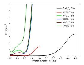
Fig.7 Optical energy gap of Cu<sub>(x)</sub>Zn<sub>(1-x)</sub> Al<sub>2</sub>O<sub>4</sub>, nano-powders (where x = 0.0 to 1.0) by using coprecipitation method non-loaded with CSs
