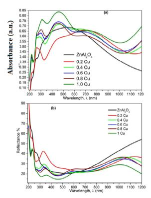
**Fig.8.** (a) Absorbance (b) Reflectance of  $Cu_{(x)}Zn_{(1-x)}$ **Al<sub>2</sub>O<sub>4</sub>** nano-powders (where x = 0.0, 0.2, 0.4, 0.6, 0.8, 1.0), using co-precipitation method loaded with carbon spheres
