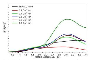
Fig.9 Optical energy gap of  $Cu_{(x)}Zn_{(l-x)}$  Al<sub>2</sub>O<sub>4</sub>, nano-powders(where x = 0.0 to 1.0) using coprecipitation method loaded with carbon spheres
