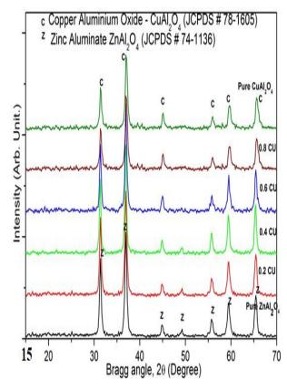
**Fig 1**: XRD patterns of  $Cu_{(x)}Zn_{(1-x)}$  Al<sub>2</sub>O<sub>4</sub> (*x* from 0.0 to 1.0 molar ratios) annealed at 1000 °C for 2 h using co-precipitation
