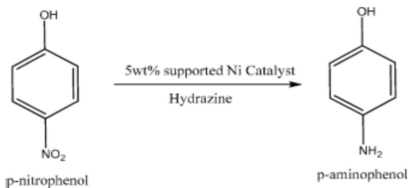
**Fig. 1.** Schematic diagram for conversion of p-nitrophenol to p-amino phenol.
