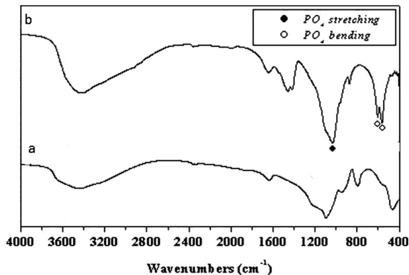
Fig. 10. IR spectra of SiO<sub>2</sub> (a) as-prepared; (b) after 14 days soaking in SBF.
