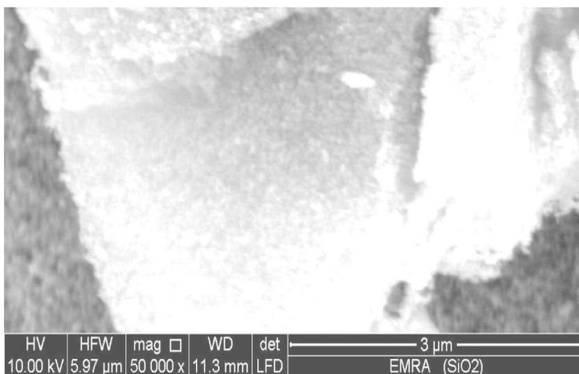
Fig. 6. SEM-image of silica with calcium carbonate calcined at 550°C.
