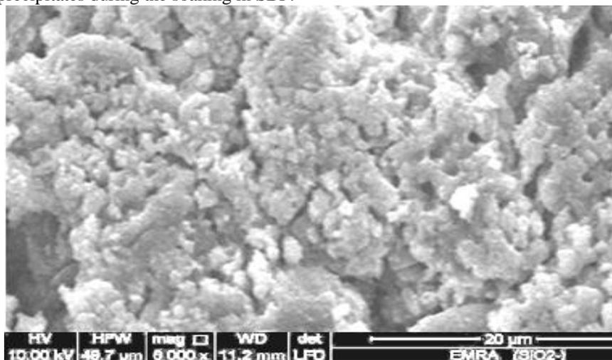
Fig. 8. SEM image shows the morphology of Apatite (AP) layer formed on silica sample after two weeks of soaking in SBF.
