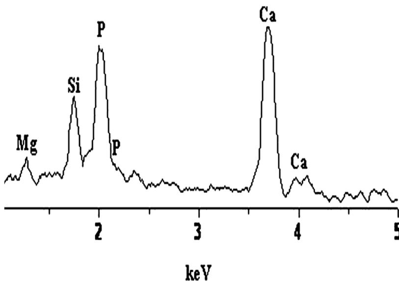
Fig. 9. EDX-spectrum of  $\text{SiO}_2$  nanoparticles after 14 days soaking in SBF.
