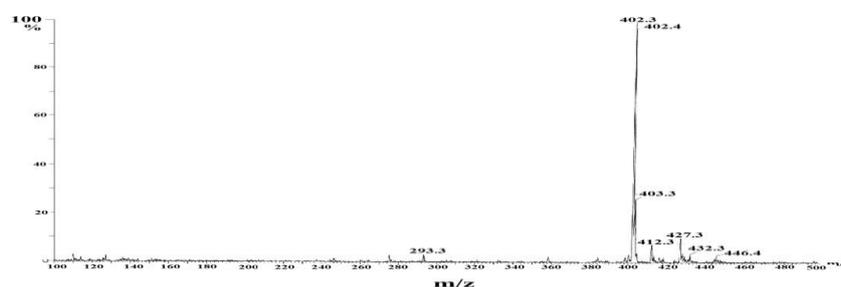
Fig. 3. Mass spectrum of MOX/ Zr complex.
