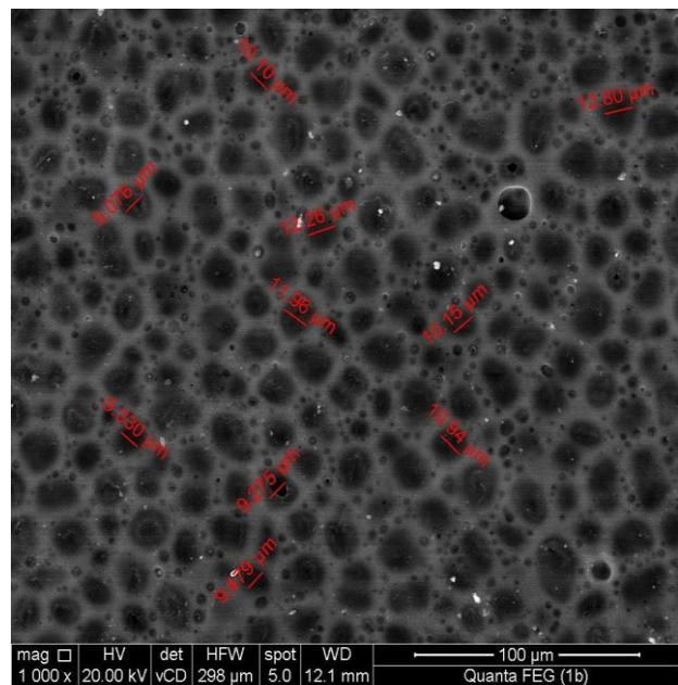
Fig. 4. SEM image of the prepared membrane using 5 wt% of PEG .
