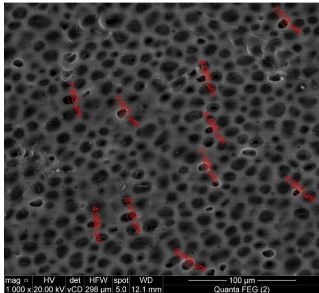
Fig. 3. SEM image of the prepared membrane using 4 wt% of PE .
