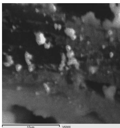
**Fig. 5.** Scanning electron micrograph of 5% Ni/  $\text{CaCO}_3$  before addition of p-nitrophenol.
