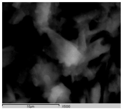
**Fig. 9.** Scanning electron micrograph of 5% Ni /  $\text{TiO}_2$  before addition of p-nitrophenol
