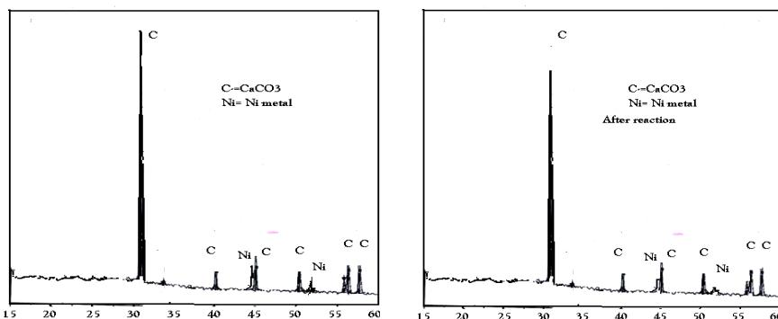
**Fig. 4.(a)**The representative XRD patterns of 5%  $\text{CaCO}_3$ - supported Ni catalyst before reaction .
