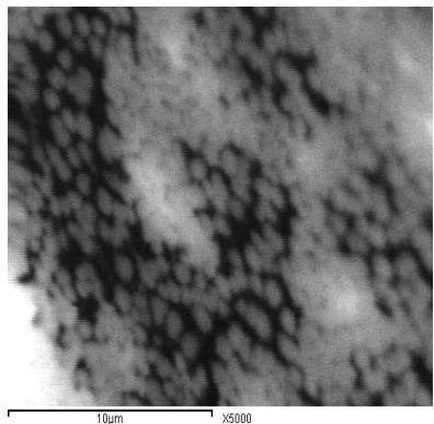
**Fig. 7.** Scanning electron micrograph of 5% Ni /  $\text{Al}_2\text{O}_3$  before addition of p-nitrophenol.
