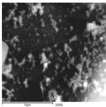
**Fig. 6.** Scanning electron micrograph of 5% Ni/  $\text{CaCO}_3$  after addition of p-nitrophenol.
