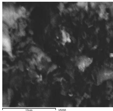
**Fig. 8.** Scanning electron micrograph of 5% Ni /  $\text{Al}_2\text{O}_3$  after addition of p-nitrophenol.
