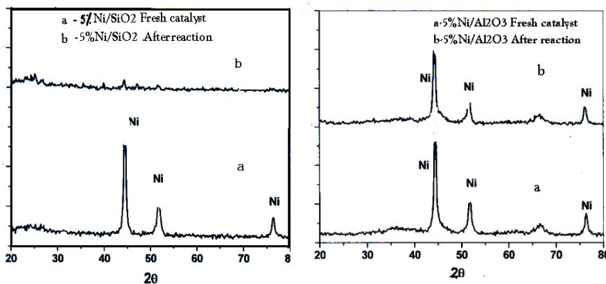
Fig. 2.The representative XRD patterns of 5% SiO<sub>2</sub>- Al<sub>2</sub>O<sub>3</sub>- supported Ni catalyst before and after reaction .
