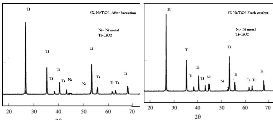
Fig. 1.(a)The representative XRD patterns of 5% TiO<sub>2</sub>- supported Ni catalyst before reaction .
