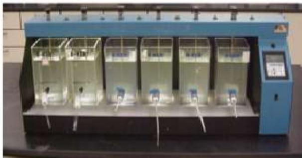
**Fig.1. Standard Jar test apparatus.**
